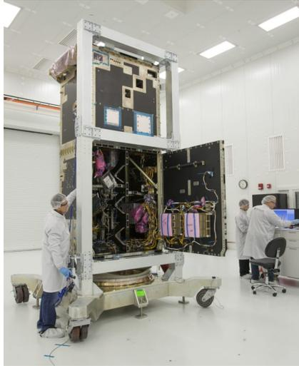
**Fig 7** CASTOR will be mounted on the MAC-200 satellite bus from Magellan Aerospace Corporation. This bus is pictured during assembly of the Radarsat Constellation Mission which launched in 2019. For more details, see §2.5.
