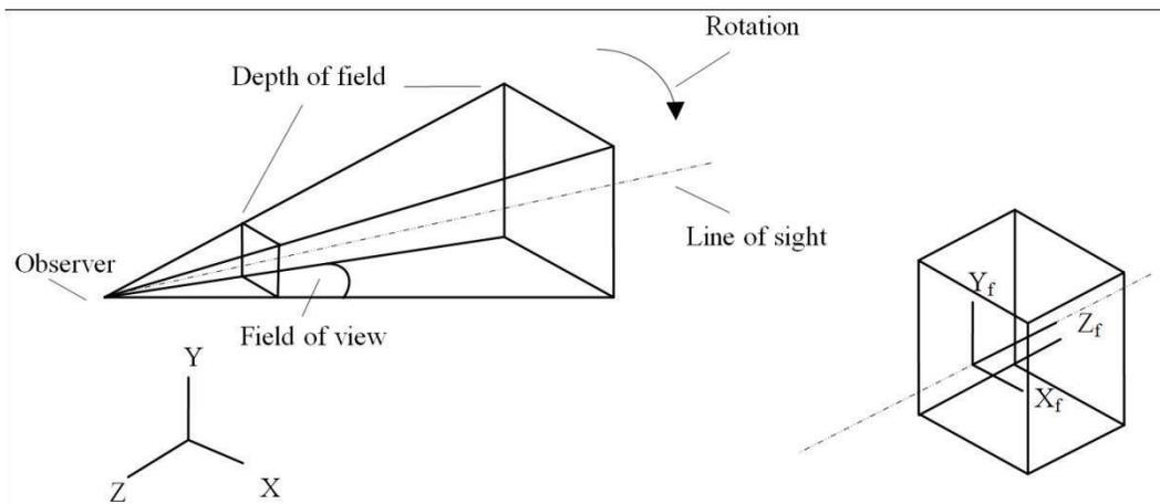
**Figure 7.** An image frustum in heliocentric space, and the rectangular frustum space. Any astronomical image is a representation of the three dimensional frustum volume defined by the observer location, the field and depth of view of the image, the line of sight, and the rotation of the image. Points in heliocentric space may be easily transformed into points in the frustum space, facilitating image-object intersection and object motion characterization.
