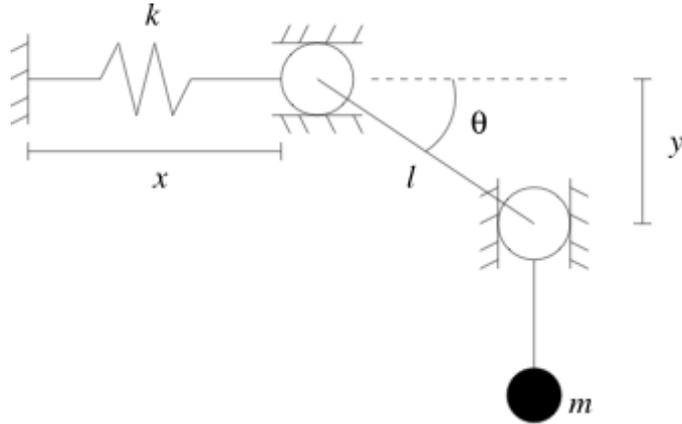
**Figure 4-6** – An arrangement of a spring, mass, and mass less pulleys.
