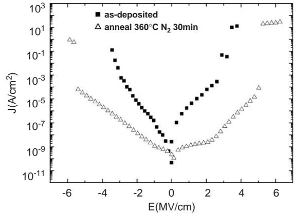
Fig. 5. Dependence of leakage current density on electric field for Sc<sub>2</sub>O<sub>3</sub> film 181 Å with an undoped amorphous Si cap layer 24.8 Å.
