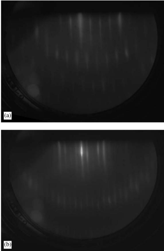
Fig. 1. In situ RHEED patterns of the  $\text{Sc}_2\text{O}_3$  film 5 nm thick showing a  $(4 \times 4)$  reconstruction showing (a)  $[4\bar{2}2]$  and (b)  $[2\bar{2}0]$  directions.
