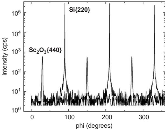
Fig. 4. Phi cone scans of Si{220} and Sc<sub>2</sub>O<sub>3</sub>{440}.
