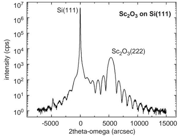
Fig. 2. Single crystal X-ray scan of the thin  $\text{Sc}_2\text{O}_3$  film along the surface normal of the Si(111) substrate.
