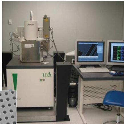
The micrograph (bottom right) shows a square array of 300nm holes on 700nm pitch written in PMMA on Si. Also shown is an array of Cr dots on Si patterned by e-beam lithography and liftoff (below).
