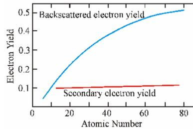
**Q:** Why do the backscattered electron micrographs, rather than secondary electron micrographs reveal the compositional contrast?
