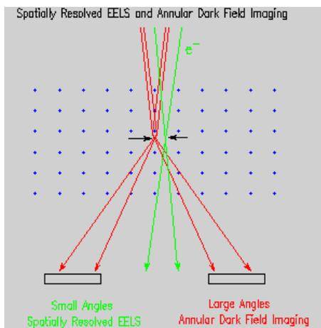
Detect only scattering at high angle, primary sensitive to the atomic number and thickness
