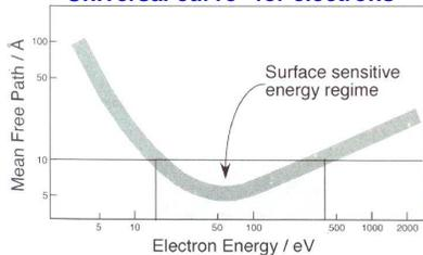
Short inelastic mean free path for electrons means that elastic scattering of electrons is **very surface sensitive**
