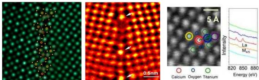
Direct Determination of Grain Boundary Atomic Structure In  $\text{SrTiO}_3$
