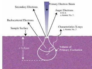
**Characteristic X-rays:** emitted when a hole is created in the inner shell of an atom in the specimen due to inelastic e<sup>-</sup> scattering, as it can recombine with an outer shell e<sup>-</sup> (EDX)
